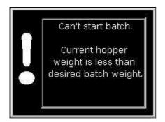
If the batching option is being used this screen will be displayed if the batching parameters can't be realised.
