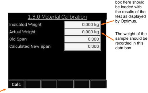
On pressing the "Calc" (f1) key Optimus will calculate a new span and display the old span.
