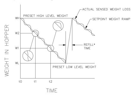
In the above diagram the desired mass rate is represented by a decreasing scheduled weight ramp. This ramp is entered into Optimus either Remotely or Locally. The slope of the scheduled weight ramp is a direct representation of the setpoint (i.e. weight of delivered material per unit of time). Increasing the setpoint increases the slope and reducing the setpoint reduces the slope.
