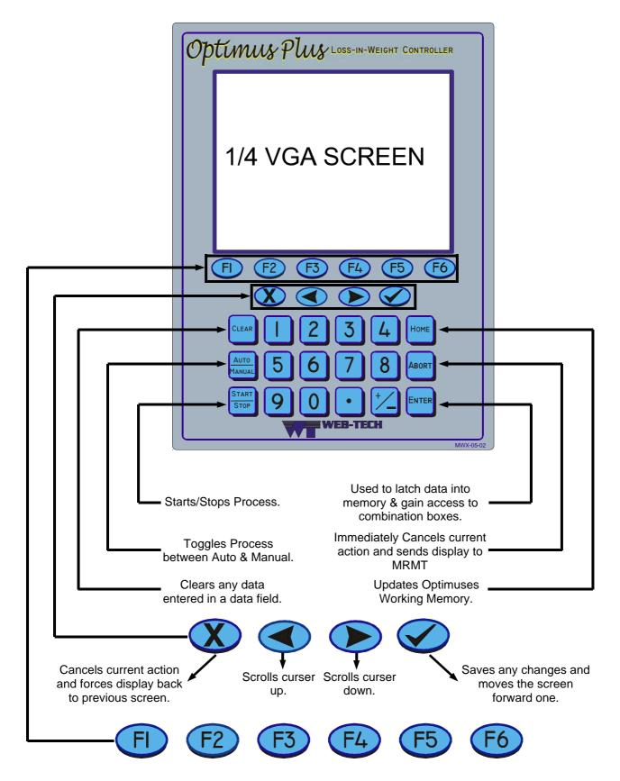
The above function (f) keys are associated with the boxed message displayed directly above the f key.
