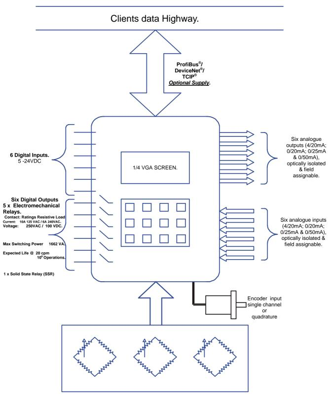
Three discrete load cell input channels, that are arithmetically summed. Negating the requirement for a summing junction box.
