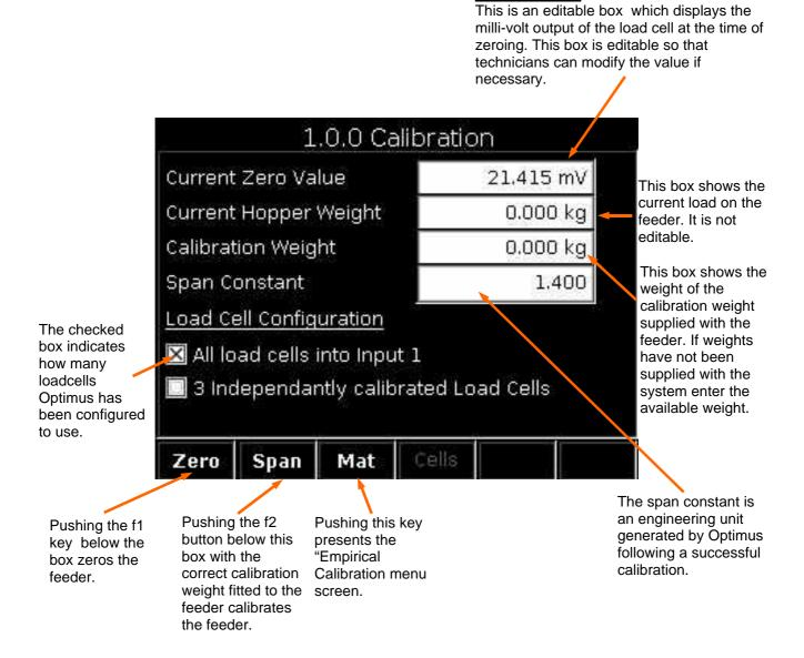
Confirm that the weight shown in the "Calibration Weight" box is correct and change if necessary. make sure the feeder is empty and there is no producer build up on the live surfaces or hopper walls. Pres the f1 button followed by the "Enter" key and the feeder will automatically zero it's self. The calibration weights should now be placed on the feeder and the f2 key pressed. Optimus will now calibrate it's self. If calibration weights are not available see detailed description.
