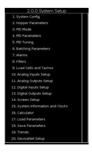
Many of the screens/menu entry points are loaded with factory defaults. These default values may not suit the process. It is therefore necessary for a commissioning engineer / technician to carefully step through each of the screens and verify that the data stored is suitable for the duty required of the feeder.
