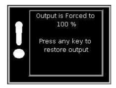
During the calibration of the analogue output current loops. The loop can be forced to 100% output. This prompt box keeps the operator informed of the loops status and provides a reminder that the previous output will be restored when any key is pressed at the end of the test.
