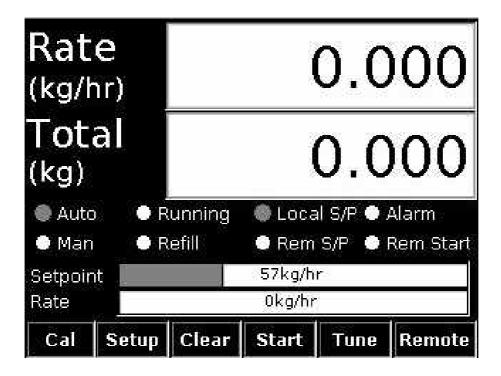
This screen is the screen that should be displayed whilst Optimus Plus is running. We call this particular screen Mass Rate, Mass Total (MRMT) and is the default screen. Take time to make yourself familiar with the data that is available on this screen and how it interacts with the keypad.
