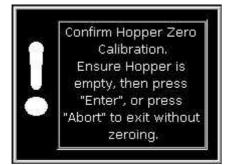
It is important that the hopper is empty prior to zeroing. This prompt confirms with the operator that the hopper is empty.
