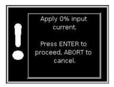
During the calibration of the analogue output current loops. The loop can be forced to 0% output. This prompt box keeps the operator informed of the loops status and provides a reminder that the previous output will be restored when any key is pressed at the end of the test.
