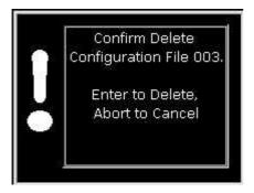
This box will appear if the user presses Delete (f2) key. It provides an escape route if the user does not wish to delete the relevant configuration file.
