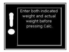
When calibrating empirically calibrating Optimus, this message box may appear if a complete data set is not provided. Weight achieved by Optimus and the weight achieved by a static scale.
