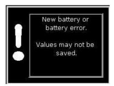
This box is displayed if the internal battery is flat or defective. It will also display this message when first switched on
