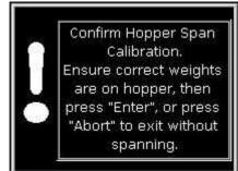
It is important that the hopper is loaded with the correct calibration weights when spanning. This message box confirms with the operator that the correct weight has been applied to the hopper.
