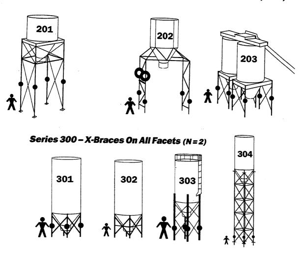
Represents typical mounting location for placement of two-sensor array. Error specifications published in this document are effective for all bolt-on products shipped after July 1, 1990.
