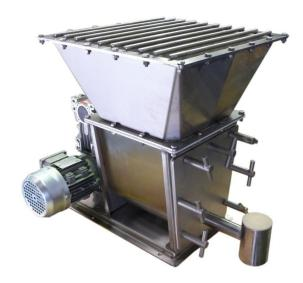
The model "VF1500" is one of Web Tech AutoWeigh's small capacity volumetric feeders, and is suitable for applications including powder and granular materials. Available in both single and twin screw configurations, accuracies in the order of  $\pm 1\%$  to  $\pm 3\%$  are achievable depending on the material bulk density consistency.
