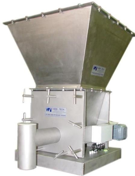
The model “VF3000” is one of Web Tech AutoWeigh’s large capacity volumetric feeders, and is suitable for applications including powder and granular materials. Available in both single and twin screw configurations, accuracies in the order of  $\pm 1\%$  to  $\pm 3\%$  are achievable depending on the material bulk density consistency.
