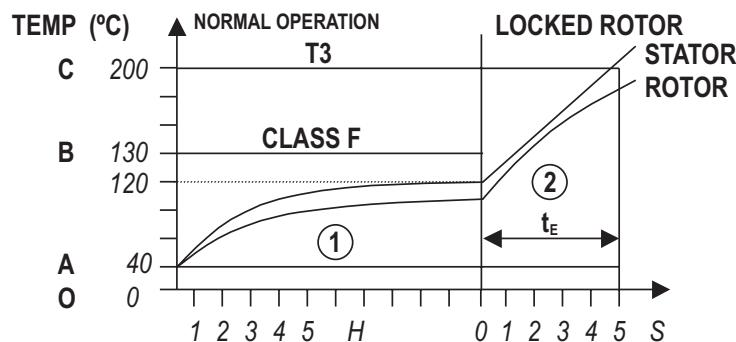
*On the chart above, the interval OA represents the maximum ambient temperature, and OB is the temperature reached under normal operating duty. In case there is any failure with further rotor locking, the condition is represented on the interval 2 of the chart. The motor temperature increases fastly up to interval OC which must be shorter than motor classification temperature T. So care must be taken to ensure motor is switched-off within time  $t_E$ .*
