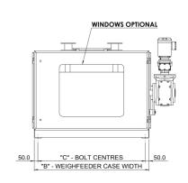
**ELEVATION WITH DOORS REMOVED**
