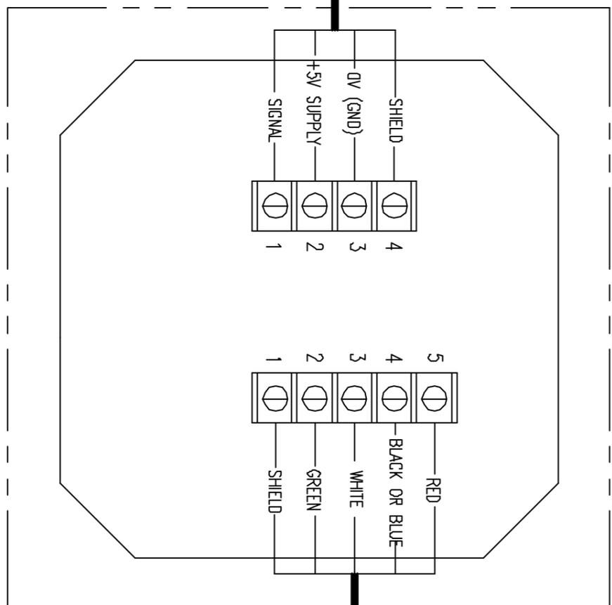
CABLE SUPPLIED BY CUSTOMER. CABLE TO BE BELDEN 3 CORE PART No. 8770 OR EQUIVALENT
