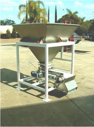
Weigh Belt Feeder, hopper and support frame.
